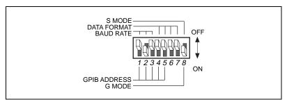
Figure 1-2. Sample GPIB Emulation Mode Switch Setting
