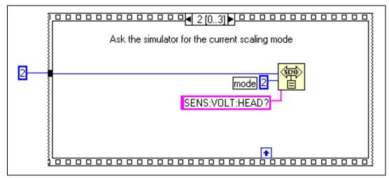
Figure 3-14. Example 3 Sequence Frame 2 Diagram
