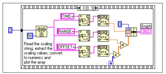
Figure 3-15. Example 3 Sequence Frame 3 Diagram
