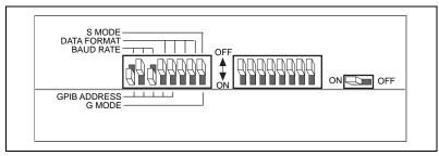
Figure 1-1. Simulator Rear Panel
