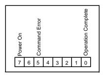
Figure 2-1. Three ESR Bits Set by the Simulator
