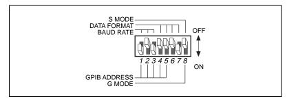
Figure 1-3. Changing the S Mode Characteristics
