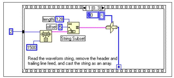
Figure 3-13. Example 3 Sequence Frame 1 Diagram
